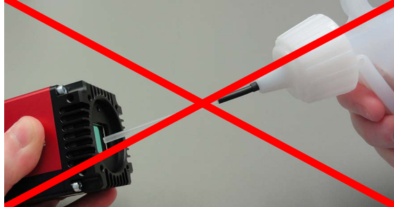
Figure 111: How not to use compressed air
