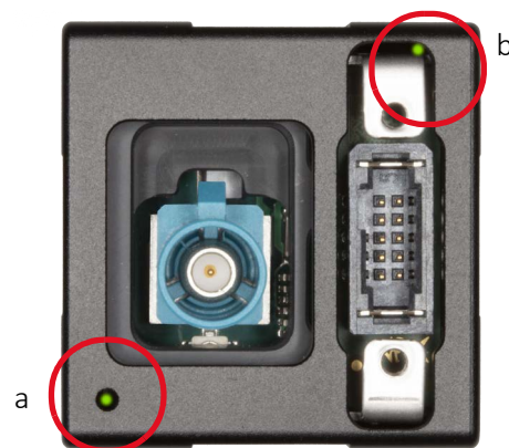
Figure 38: External LED (a) and internal LED (b) on a Coax model
