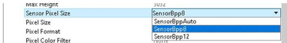
By default, sensor pixel size is "SensorBppAuto" and should follow the adjustment of pixel size.
