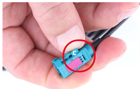
Figure 25: Pressing down the latch (c) of the HSD STP connector
